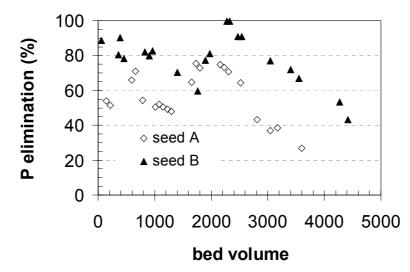
Figure 3 Comparison of the P-elimination efficiency of seed materials A and B (5 wt-%) in expanded bed experiments.
