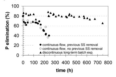
**Figure 2** Comparison of discontinuous long-term batch (HRT: > 2 h) and continuous-flow stirring reactor experiments (HRT: 2 h) and impact of previous removal of suspended solids regarding the P-elimination efficiency of seed material B (5 wt-%); SS: Suspended solids.
